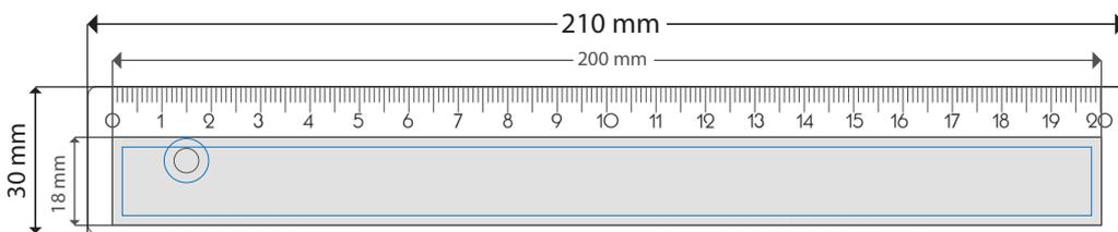
○ Ø 5 mm – POS Mitte 20 mm v. linker Kante, 15 mm v. unterer Kante
